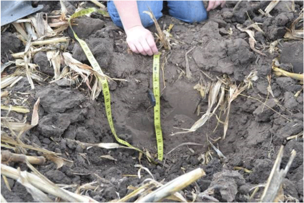
Figure 1. Digging a small hole with a spade is the best way to learn about the soil's natural and unnatural layers, such as compacted layers. Use a knife to feel for any unusually dense layers, and a tape measure to determine the depth of the layer. Photos courtesy of DeAnn Presley, K-State Research and Extension.
