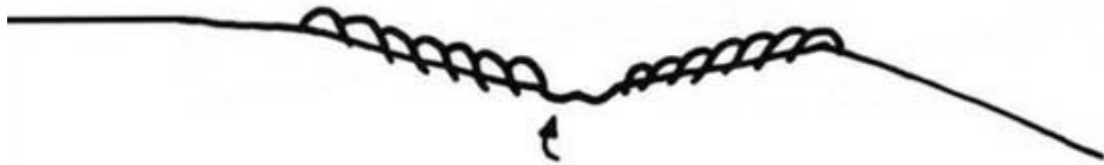
Figure 2. Enlarging and widening the terrace channel. The arrow indicates the two dead furrows meeting at the center of the channel. Image from K-State Research and Extension.
