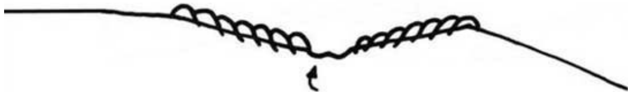
Figure 2. Enlarging and widening the terrace channel. Arrow indicates the two dead furrows meeting at the center of the channel. Image from K-State Research and Extension.
