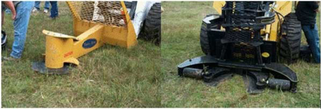
Figure 2. Turbo saw (left) and hydra clip (right).
