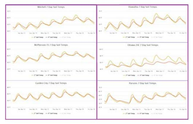
Figure 2. 7-day soil temperatures (2- and 4-inch soil depth) for Hiawatha, Ottawa, Parsons, Mitchell, McPherson, and Garden City. 2-inch depth represented by yellow line; 4-inch depth represented by orange line. Graphs produced by the <u>Kansas Mesonet</u>.
