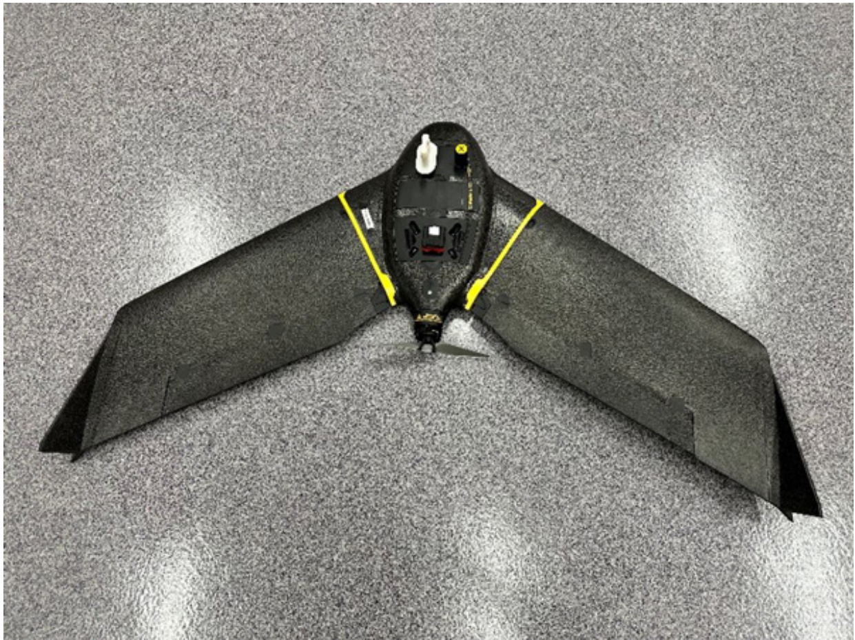
Figure 1. Fixed wing drone with multi-spectral sensor that can be used for agricultural field scouting. Photo by Deepak Joshi, K-State Research and Extension.
