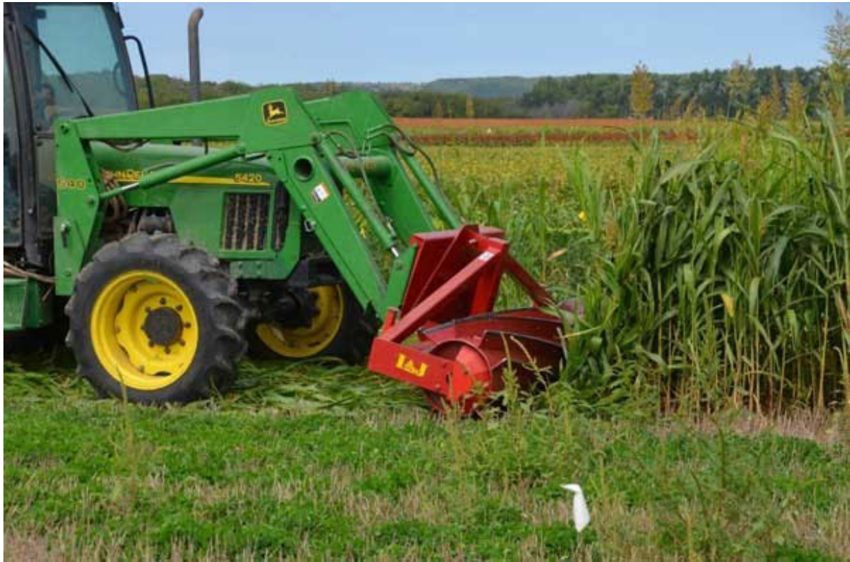
Figure 2. Roller crimper being used to terminate a sorghum-sudan grass summer cover crop. Photo by Peter Tomlinson, K-State Research and Extension.
