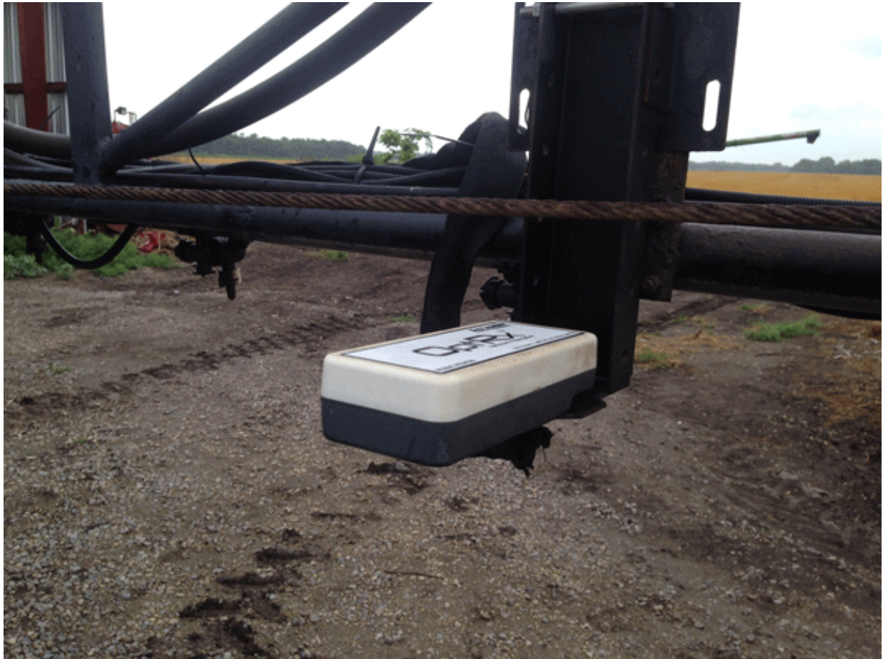
Figure 3. Ag Leader OptRx sensor mounted on boom. Photo by Ray Asebedo, K-State Research and Extension.
