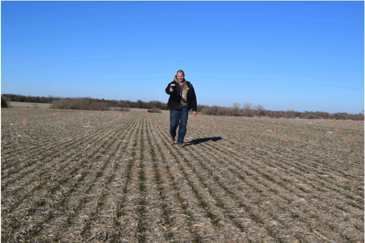
Figure 5. Using handheld GreenSeeker sensor prior to topdressing wheat. Photo by Dave Mengel, K-State Research and Extension.
