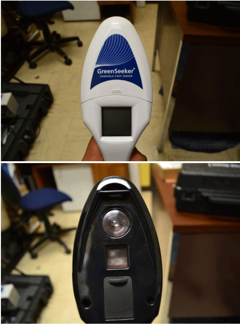
Figure 4. Top and bottom view of Trimble GreenSeeker sensor. Photo by Ray Asebedo, K-State Research and Extension.
