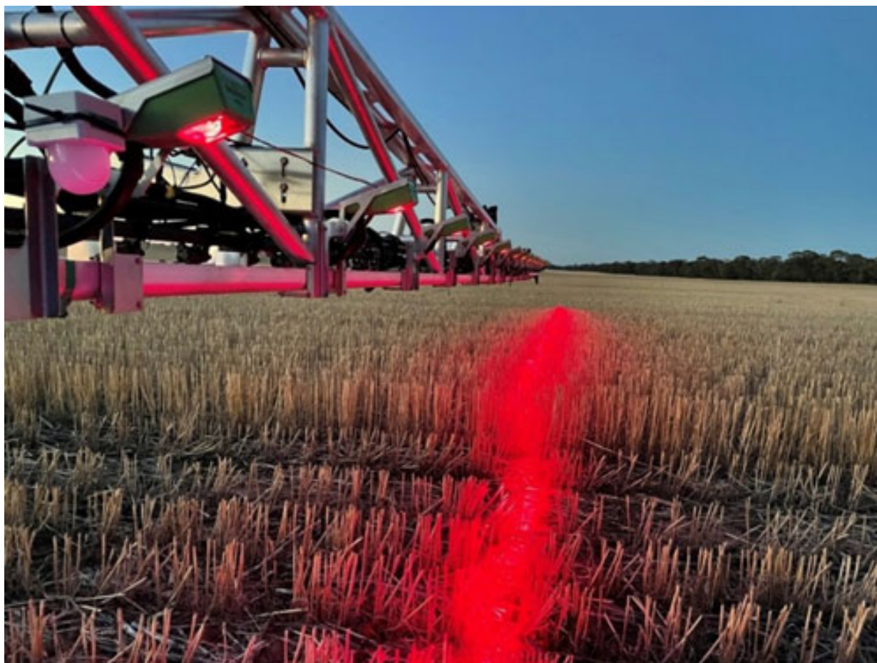
Figure 1. WEED-IT Quadro Red emits red LED lighting and detects returning chlorophyll fluorescence from plants. Image Courtesy Weed-IT ( https://weed-it.com/what-is-weed-it/ ).
